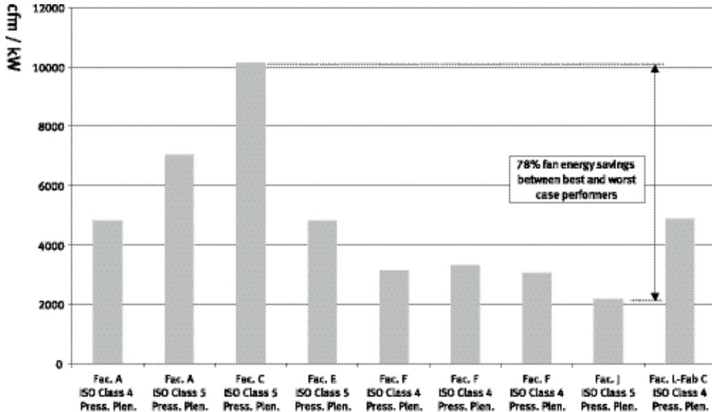
The figure above shows the variation in performance between pressurized plenum recirculation air systems as found in the LBNL Benchmarking project. The worst performer was the cleanroom in Facility J at 2185 cfm/kW. The best performer was the cleanroom in Facility C. The best performer saved 78% of the fan energy of the worst performer.
