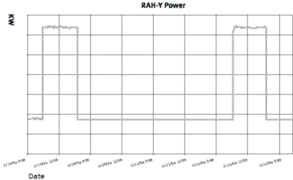
The figure above shows the reduction in fan power for a cleanroom where a timer was used to set back airflow when the cleanroom was unoccupied at night and on weekends. The air change rate was reduced from 594 ACH to 371 ACH to achieve this reduction. Another case study showed similar reduction in fan power as shown in Figure 3 below.
