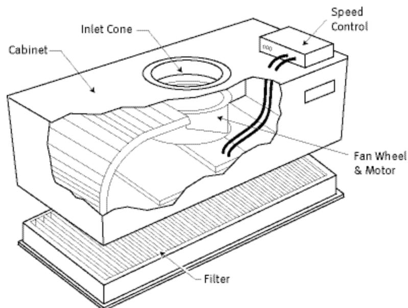
FFU systems are required for many specific applications; however, FFU systems tend to be less energy-efficient than pressurized plenum systems for recirculating air in a cleanroom (Figure 2).
