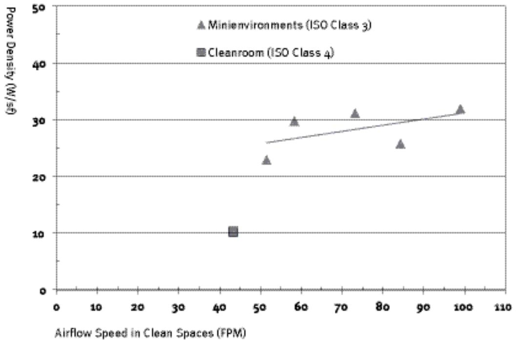
Corresponding to the operating airflow speeds that ranged from 50 fpm to 100 fpm, and power density of the minienvironments ranged from 26 W/sf to 32 W/sf with an average of 28 W/sf (Figure 3). Lower power density generally indicates better energy performance to achieve the desired cleanliness within the minienvironments.
